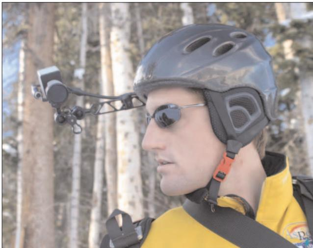
For the paraglider shots, Lenzo devised a POV system with an Ikegami HDL-20 camera and a small Canon 7 mm lens, and tethered it to the same Sony HDW-250 VTR packed into the Kata backpack. He monitored through a tiny heads-up display rigged under his helmet.
