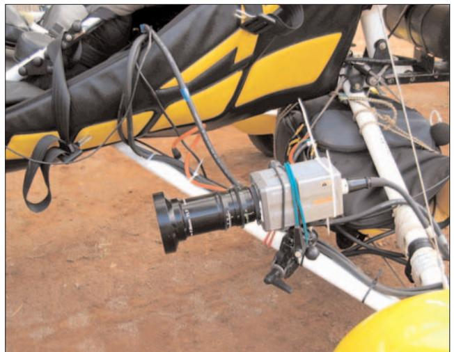
Lenzo used a Sony DXC-H10 HD camera fitted with a Canon FJ5 5 mm prime HD lens, and occasionally a Canon IMS-20 image stabilizer, to send a signal to a Sony HDW-250 HDCAM VTR packed into a Kata Panda camera backpack. Camera operators monitored the signal and framed shots through an ERG Ventures HDM-EV20D LCD monitor. On the right, the camera and VTR bag are mounted on an ultralight in the first POV position.
